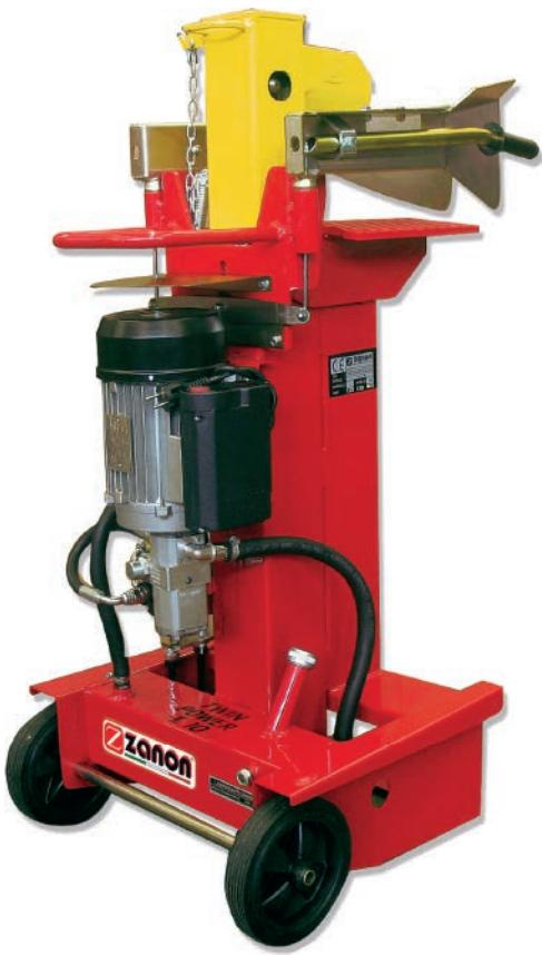
**Use:** the SLE-10 log splitter has an 10 ton thrust and can split logs of various sizes, up to 57 cm in height. It is equipped with wheels for moving it, a large reinforced working table, an automatic adjustable "end-of-stroke control" system, and special safety devices that protect the user.
